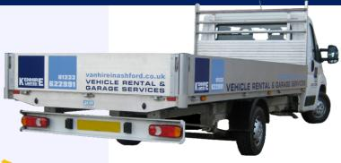
The longest in our range of 3.5 ton trucks, the extra long wheelbase Relay Dropside is ideal for scaffolding companies, with a 4.8 meter load length and full width over cab gantry
